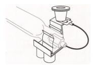
To ensure proper installation, each SPECTRAMATCHTM lamp comes with detailed instructions, a cotton glove and alcohol wipe. Make sure the horseshoe-shaped spade connectors at each end of the lamp (see diagram) are securely fastened by the thumbscrews. A loose connection can cause arcing, overheating, early lamp failure and permanent damage. A discolored connection may be a sign of damage, so contact OLEC if you have any questions.
