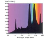
Spectral Output Diazo Model L1280 Wattage 2,000-8,000 Light Source AL83
