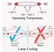
air at the hottest part of the lamp, OLECs unique Servo-Controlled Cooling system monitors lamp temperature and sends the optimum amount of cool air in proportion to the demand. This ensures consistent exposures and longer lamp life.
