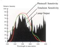
fight spectrum of the material to be exposed. This Spectral Matching results in the fastest exposure possible, at each wattage level. OLECs SPECTRAMATCH™ colored lamp ends correspond to the lamp's spectral output to help you choose the correct lamp for your application.
